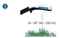
Hold the sensor over the crop canopy and then pull the trigger. The sensor should be held 24 - 48" above the crop.
