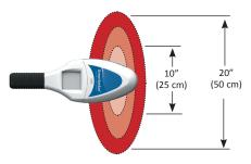
To obtain a reading representing a larger area, walk with the sensor while keeping the trigger engaged and maintain a consistent height above the target. The display updates continuously, but accumulates multiple readings and provides an average when the trigger is released. The maximum measurement interval is 60 seconds.
